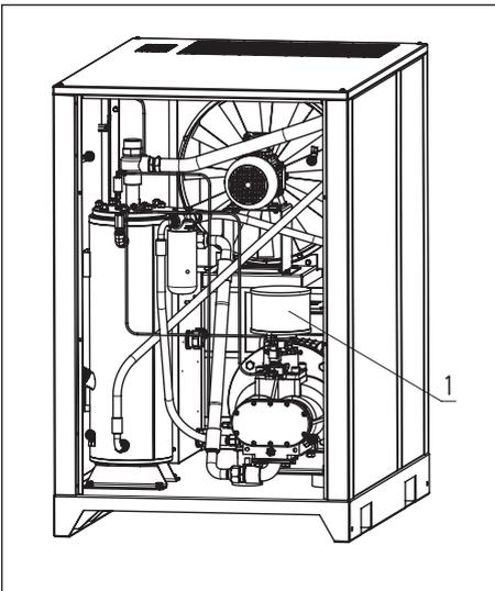
The air filter (1) is attached to the compressor's intake valve. In order to replace it, open the front side panel, loosen the clamp securing the filter. Remove the contaminated filter, and detach the clamp from it. Set the new filter in its place and fit into place with the clamp.
