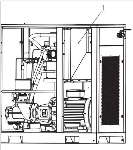
In order to access the radiator (1), open the front or right panel. Regularly clean the radiator in order to maintain its cooling efficiency at an acceptable level. Remove any dirt particles from the radiator using a fibre brush, then aim a jet of compressed air at the radiator from the bottom to the top; the jet should be held at an approximate 90° angle to the plane of the radiator.
