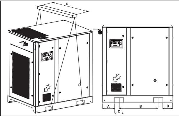
For transport with a forklift truck, use the rigging holes in the frame. The compressor has slotted rigging holes with width C – fig. 3.1. Move the compressor carefully.
