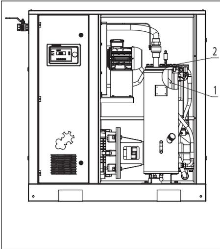
The separating component (1) is located within the separator tank. Open the front panel in order to change it. Unscrew the bolts (2) and carefully remove the top cap of the tank. Disconnect hoses if they make it difficult to remove the cap. Remove the spent separator and install a new one in its place. Refasten the tank cap.
