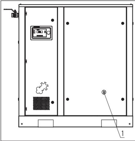
Check oil level on a daily basis. In order to access the oil level, stop the compressor and remove the front side panel. The oil level in the compressor should be checked visually with the oil level glass (1) when the compressor has stopped. The surface of the oil must always be visible in the sight glass. If no oil is visible in the sight glass, the oil level is low and needs to be topped up. Using belt tension gauge, check the tensile force of the compressor belts.
