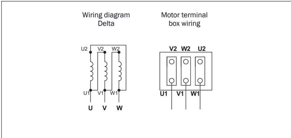
Fig. 2.6.2 Electric motor wiring diagram for DV30-55
