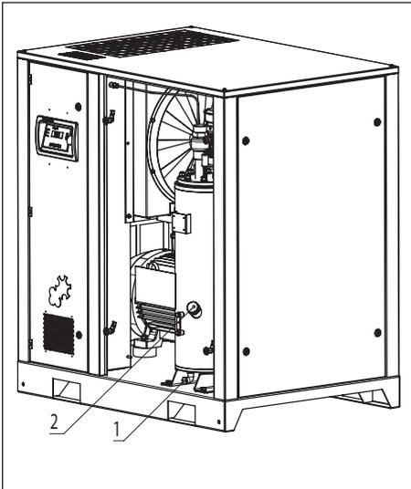
Open the front panel and turn the fill plug (2) one revolution in order vent system pressure. Remove the fill plug. Remove plug from the drain valve (1) at the bottom of the Air-Oil separation tank. Drain the oil into a dedicated vessel from the separator tank after opening the drain valve. Fill the Air-Oil separation tank with oil until it is level with the middle of the sight glass. Refit and tighten the drain valve plug and the fill plug.
