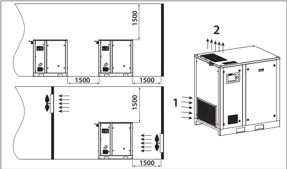
Fig. 3.4 Installation facility proposal D11 – D22
