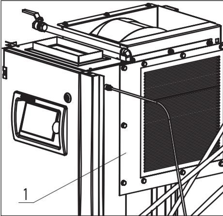
In order to access the radiator (1), open the front or right panel. Regularly clean the radiator in order to maintain its cooling efficiency at an acceptable level.
