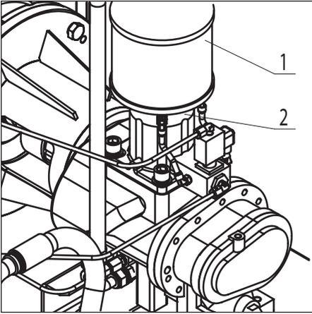
The air filter (1) is attached to the compressor's intake valve. In order to replace it, open the front side panel, loosen the clamp (2) securing the filter. Remove the contaminated filter, and detach the clamp from it. Set the new filter in its place and fit into place with the clamp.
