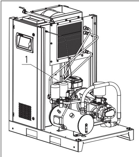
Fig. 5.5.1 Changing air-oil separator D11 - D15
