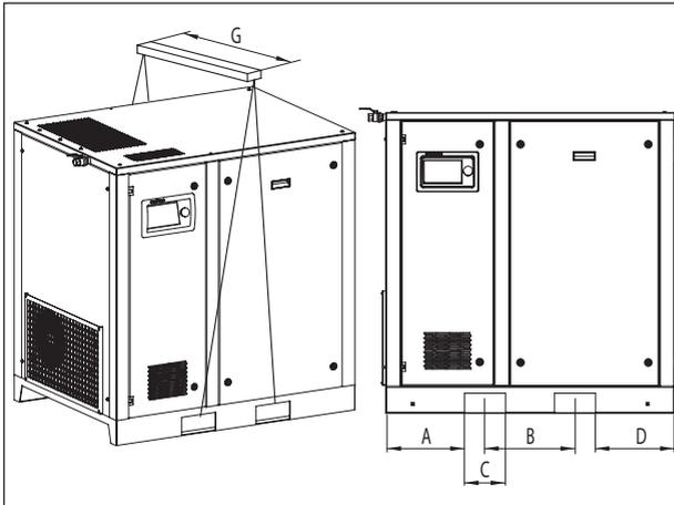
For transport with a forklift truck, use the rigging holes in the frame. The compressor has slotted rigging holes with width C – fig. 3.1. Move the compressor carefully.
