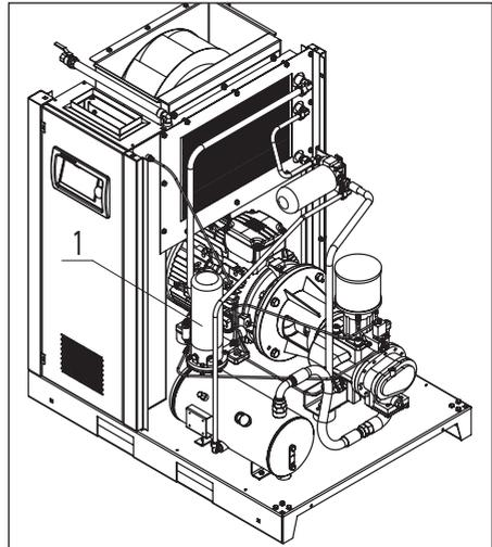
Fig. 5.5.2 Changing air-oil separator D18 - D22
