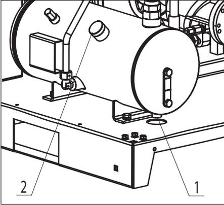
Open the front panel and turn the fill plug (2) one revolution in order vent system pressure. Remove the fill plug. Remove plug from the drain valve (1) at the bottom of the Air-Oil separation tank. Drain the oil into a dedicated vessel from the separator tank after opening the drain valve. Fill the Air-Oil separation tank with oil until it is level with the middle of the sight glass. Refit and tighten the drain valve plug and the fill plug.
